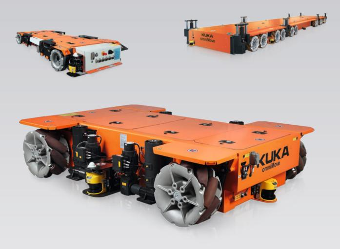
Now even XXL components can be set in motion. The KUKA omniMove maneuvers aircraft, wind power plant and rail vehicle components to the exact location where they are required for the production process. e-mobility and KUKA intelligence make the production process quicker and more flexible than ever before.
