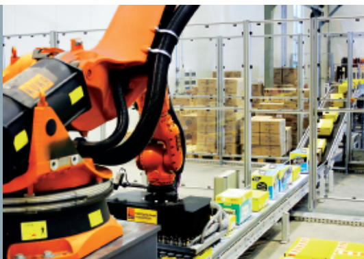
An "order picking" KUKA robot puts together shipping packages according to size and weight
