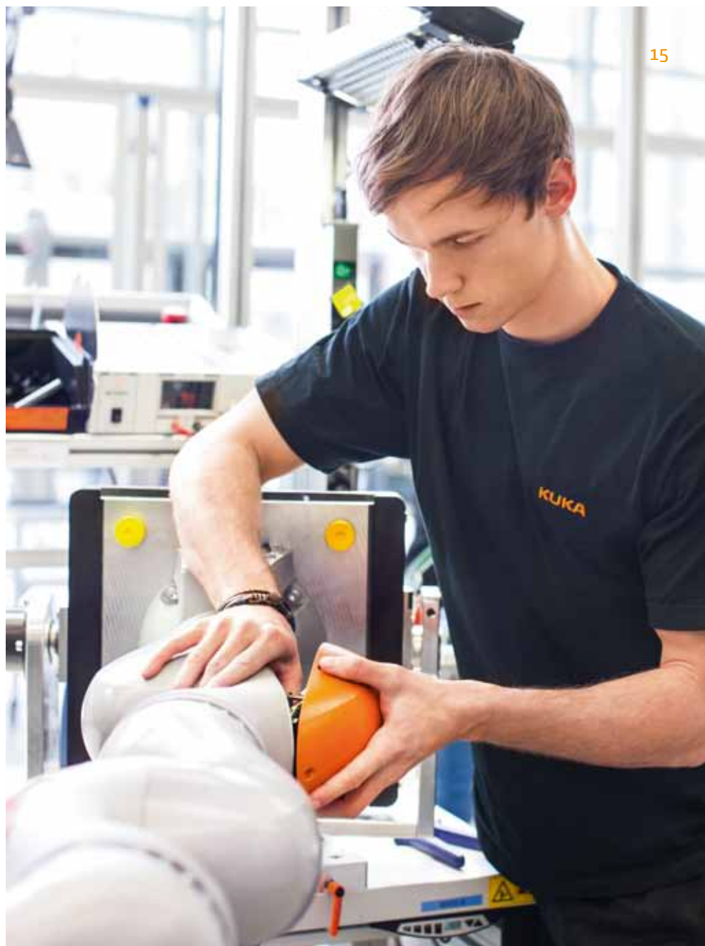
FROM THE LEFT: the LWR is assembled and wired in the final assembly area.
