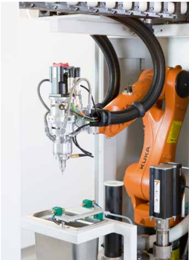
A KR AGILUS installed in a compact dosing cell at RAMPF in Baden Württemberg, Germany, occupies very little space as it applies the correct doses for foaming, casting, gluing and sealing operations.
