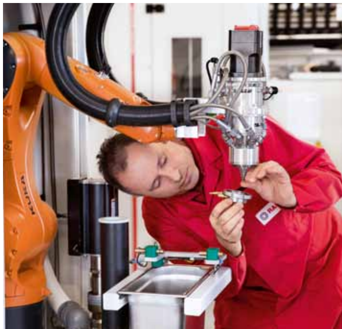
A KR AGILUS installed in a compact dosing cell at RAMPF in Baden Württemberg, Germany, occupies very little space as it applies the correct doses for foaming, casting, gluing and sealing operations.
