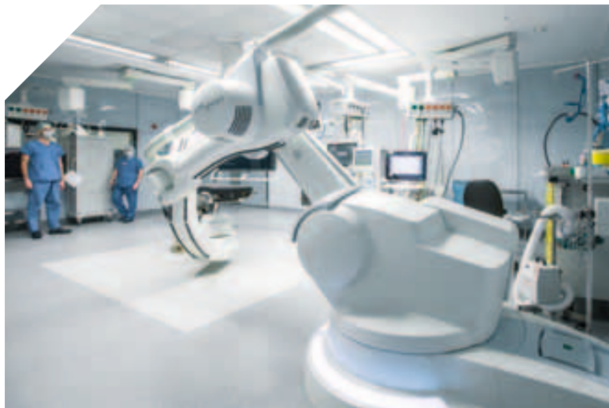
TOP AND RIGHT THE ROBOT INTEGRATED IN ARTIS ZEEGO FROM SIEMENS HEALTHCARE ENABLES THE PHYSICIAN TO POSITION THE C-ARM AROUND THE PATENT.
