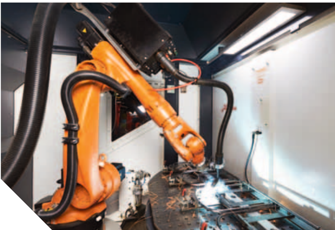
LEFT QUICK AND ACCU- RATE – THE INERT GAS WELDING PROCESS FOR JOINING STROLLER COMPONENTS
