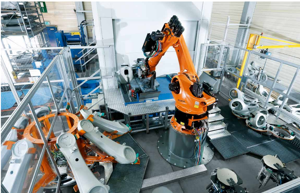
Machining center from Burkhardt + Weber, automated with a KR 500 in KUKA's in-house production.
