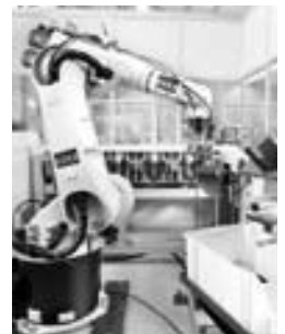
KUKA robot builds fuel cells at ZSW in Ulm.
