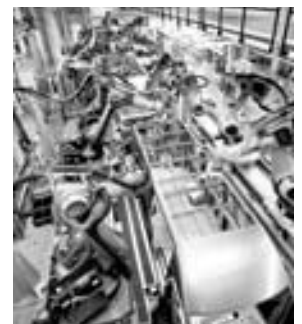
Spot welding in automotive.
