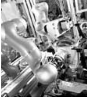
KUKA's lightweight robot assembling rear axle differentials for cars.
