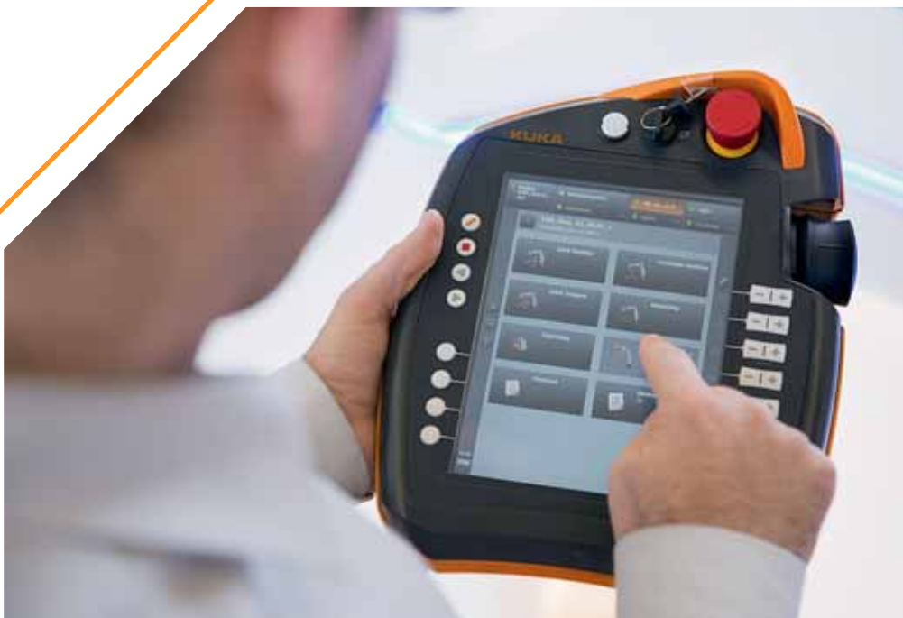
ROBOTS CAN BE EASILY AND INTUITIVELY OPERATED USING THE KUKA SMARTPAD AND ITS REDESIGNED USER INTERFACE.
