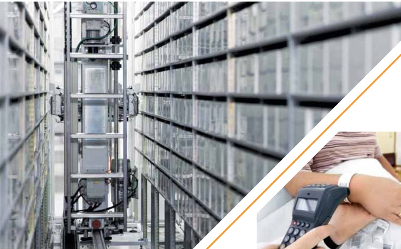
LEFT: INTERIOR VIEW OF THE BOXPICKER STORAGE SYSTEM FOR HOSPITAL PHARMACIES
