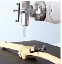
Orthopedic surgery: Thanks to its stable design and construction, as well technology and safe human-robot as its high stiffness, the LBR Med is suitable for bone surgery. Open-source of prototypes and the integration of navigation cameras.
