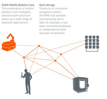
Operator The operator is relieved of monotonous, nonergonomic tasks and can concentrate on important processing steps.
