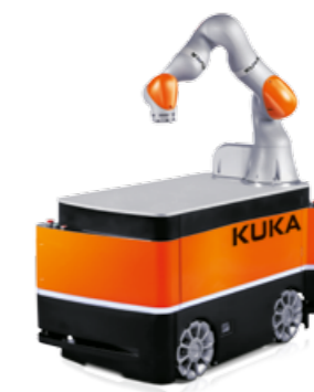
KMR iiwa An intelligent lightweight: the KMR iiwa combines the strengths of the sensitive lightweight robot LBR iiwa with a mobile, autonomously navigating platform.
