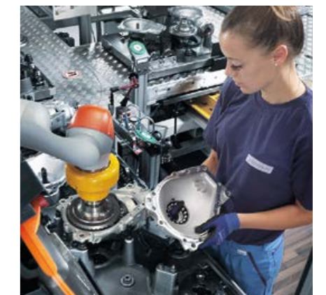
Human operators and robots collaborate to install differential cases for front-axle transmissions.
