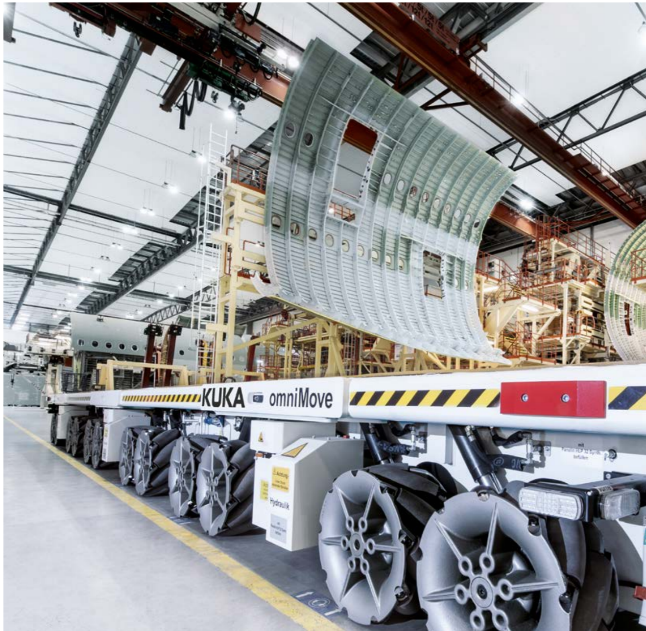
KMP omniMove Maneuvering huge components simple and safely on site: the KMP omniMove at the Airbus plant in Hamburg
