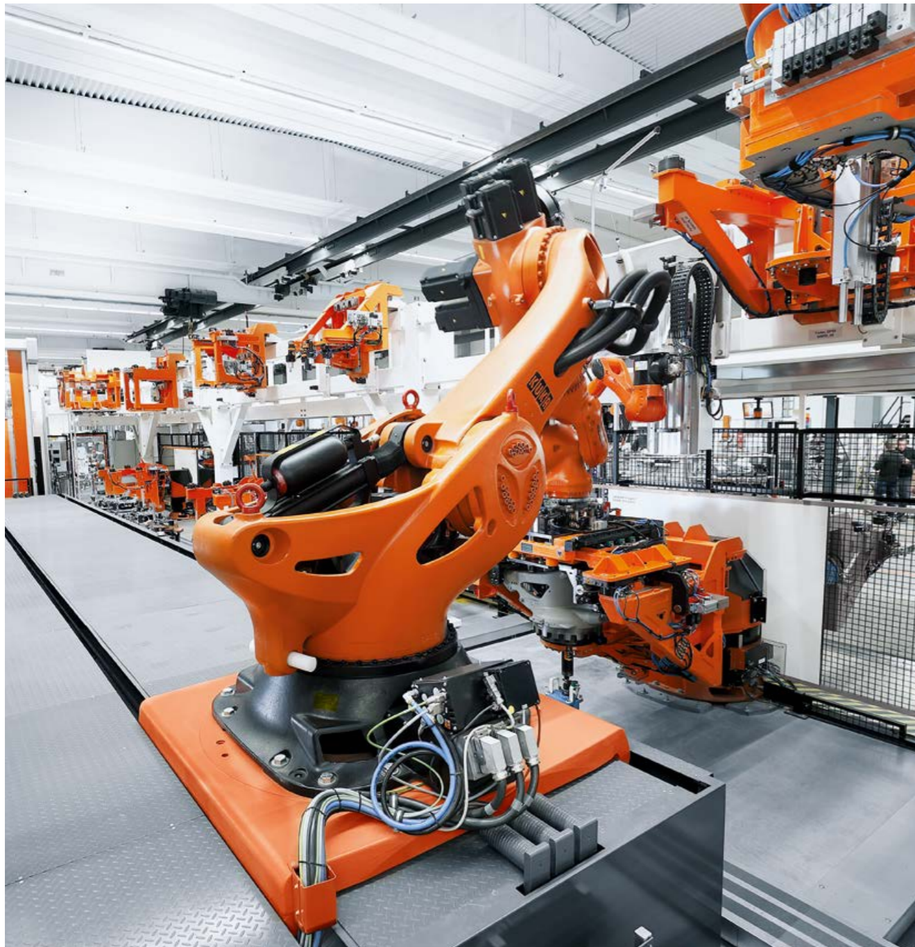
The KR titan on a linear unit in a perfect workflow with the KR AGILUS
