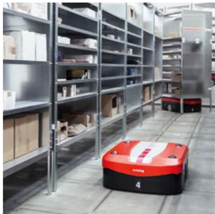
CarryPick Designed to be modular and multifunctional, CarryPick from Swisslog consists of mobile racks and automated guided vehicles for goods-to-person picking.
