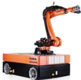
KMR QUANTEC Intelligent robotics right where it is needed: the mobile industrial robot KMR QUANTEC stands for precision transport of even the heaviest components.
