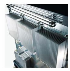
Especially low-maintenance – without filter mats. The passive heat exchange system of the KR C4, with separate air circulation in the inner and outer zones of the controller, allows low-maintenance operation even in dusty environments. Entirely without filter mats.
