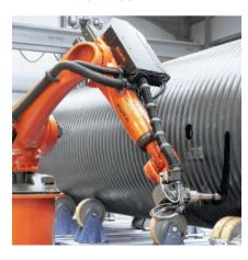
In the system: a space-saving KR AGILUS positions itself and accesses the assembly fixture from underneath
