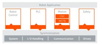
Four dedicated control modules in one control system. The KR C4 concept is revolutionary. For the first time, RobotControl, MotionControl and LogicControl are seamlessly and interactively integrated with control modules for Safety and CNC. Automation solutions based on the KR C4 are thus considerably more intelligent, flexible and scalable.
