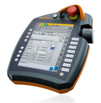
Robot operation made easy: The KUKA smartPAD brilliantly demonstrates, on a large, high-resolution antireflection touch screen, just how simple robot operation can be. Intelligent, interactive dialogs proelements that are currently required. This makes work easier, faster, more efficient and simply smarter all-round.
