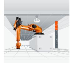
More space for your success: the virtual protected space. KUKA robots monitor their workspace by means of safe software. This means that they can also be operated in confined spaces, for example under craneways or in facilities with low ceilings.
