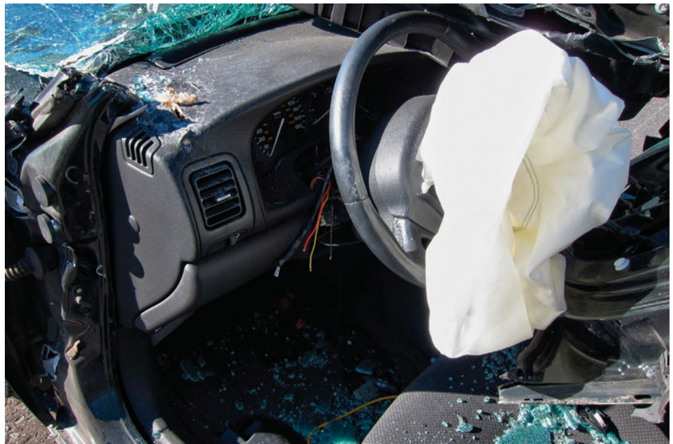
FIGURE 1-12 Lift the collapsed air bag to note whether or not there is a deformity of the steering wheel. (Courtesy of Olivier Le Queinec, Shutterstock.com)
