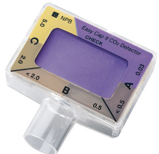
FIGURE 5-13 Colorimetric \text{CO}_2 detector. (Image used by permission from Nellcor Puritan Bennett LLC, Boulder, Colorado, doing business as Covidien)
