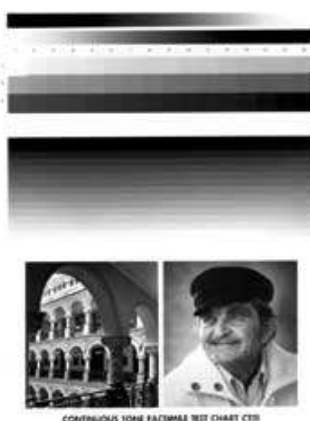
Test Chart No. 5: Continuous tone facsimile test chart CT01 (ITU-T Recommendation T.22)
